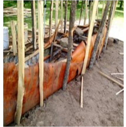
The bark is formed into shape around the frame and held in place with stakes.
