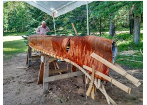
The bark has had boiling water poured on to soften it at the ends, and these wooden "clothespins" hold it in the desired shape to harden into place.
