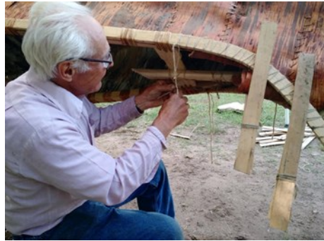
Jack is sewing the gunwales. The bark sides are sandwiched between 2 layers of wood.
