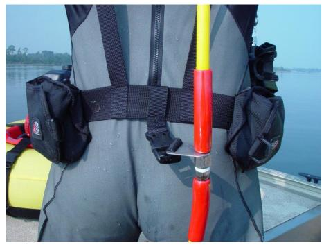
There are two types of weights used on a weighting system: hard and soft. Hard weights are solid lead pieces in various sizes, usually notched on opposite ends to allow threading onto a conventional weight belt. They are rarely used anymore. Soft weights are also lead, but they are tiny pellets encased in pouches, in various weight sizes, that fit into pockets on weight belts or weighting systems.
